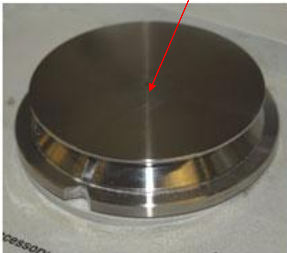
Figure 11.27 – sampling equipment for use with ATR technology
