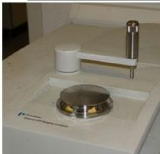
Figure 11.27 – sampling equipment for use with ATR technology
