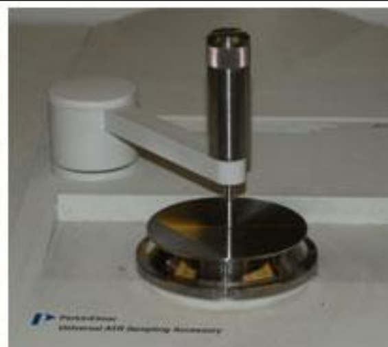
Figure 11.27 – sampling equipment for use with ATR technology
