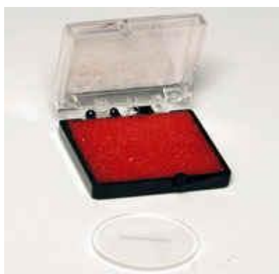
Eyepiece graticule with evenly spaced markings
