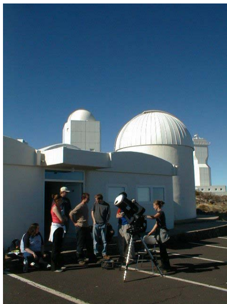
Figure 2 Astronomy students carrying out solar photographic measurements using an LX200 telescope with a solar filter
