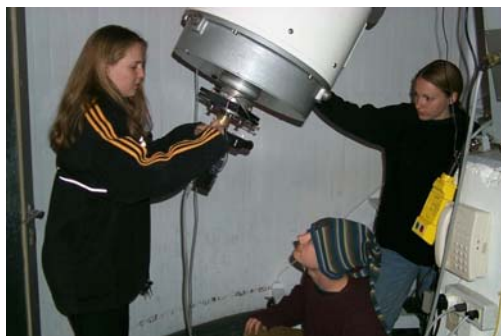
Figure 1 Astronomy students attaching a ST-6 CCD camera to the 0.5m Mons telescope
