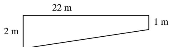
*Solution: One side has a length of 1 m, and the other 2 m. Their average is 1.5 m. This average, multiplied by the length of 22 m, gives the area as  $33 \text{ m}^2$ .*
