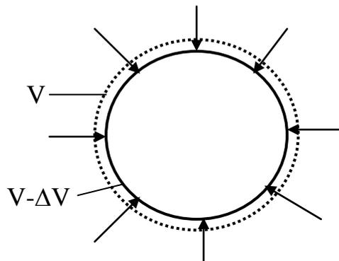
This sort of situation would occur, for example, if the body were taken down to the sea bed. The weight of water above creates a high pressure, known as hydrostatic pressure, which acts in all directions.
