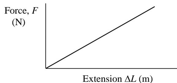
This is an example of Hooke's Law, which states that the change in length of a material is proportional to the applied force. The stretching of the material sets up internal forces which balance the applied external force. Most solids obey Hooke's Law, at least for moderate loads. We can express Hooke's Law mathematically by:
