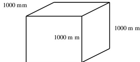
$$\text{Volume} = 1000 \text{ mm} \times 1000 \text{ mm} \times 1000 \text{ mm} \\ = 1\,000\,000\,000 \text{ mm}^3 \text{ (or } 1 \times 10^9 \text{ mm}^3)$$
