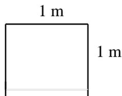
$$\text{Area} = 1 \text{ m} \times 1 \text{ m} = 1 \text{ m}^2$$
