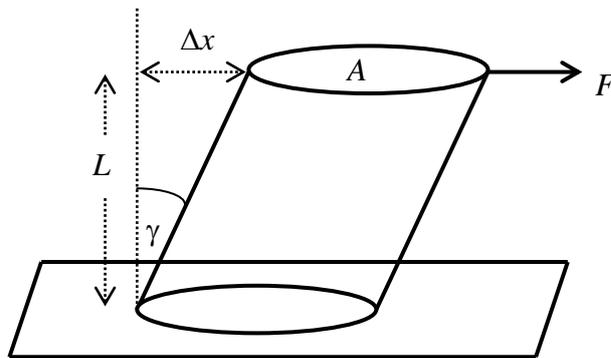
The figure shows the response of a material to a shear stress. Imagine a cylinder of length  $L$  and cross sectional area  $A$ . One end is firmly attached to a surface, the other end is subjected to a force  $F$  parallel to the face. The shear stress is given the symbol  $\tau$  (Greek tau):
