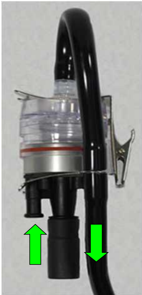
Figure 2.53 – cyclone personal sampler
