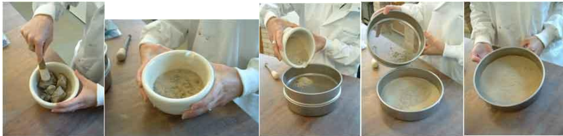
Fig 2.18 – grinding and sieving a dried sample of soil
