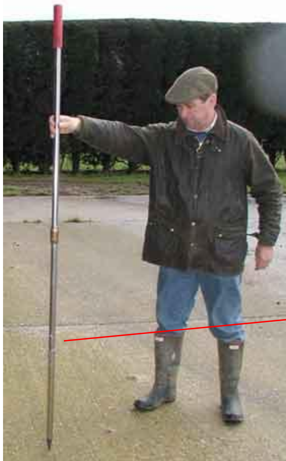
Fig 2.4 – spear device for vertical sampling of grains
