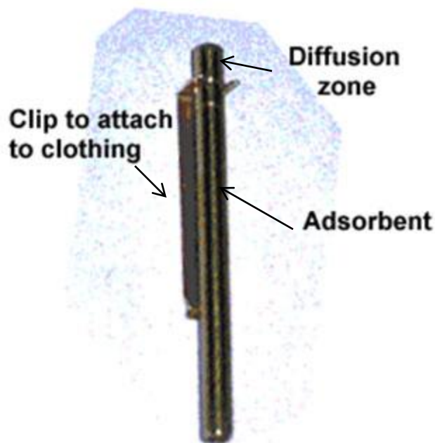
Figure 2.48 – stainless steel passive sampler
