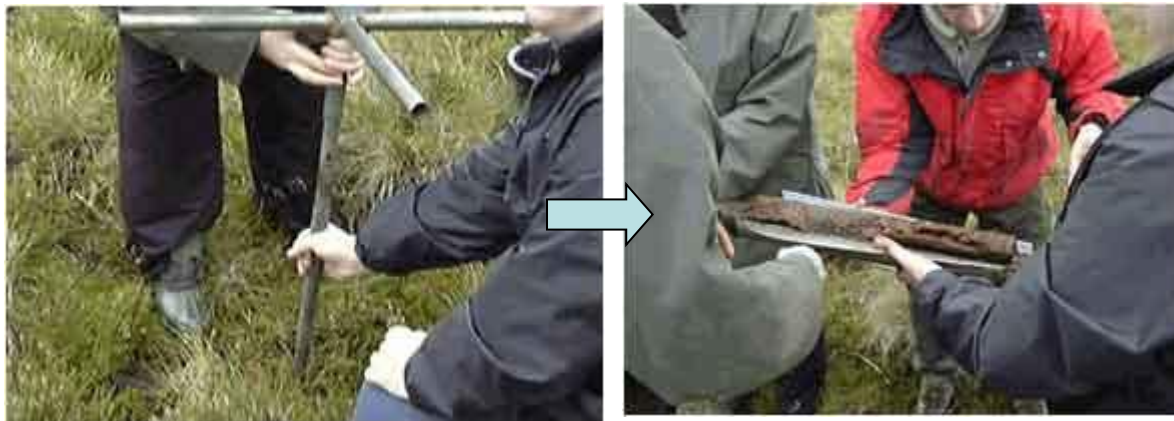
Fig 2.19 – corer sampler being used to sample peat
