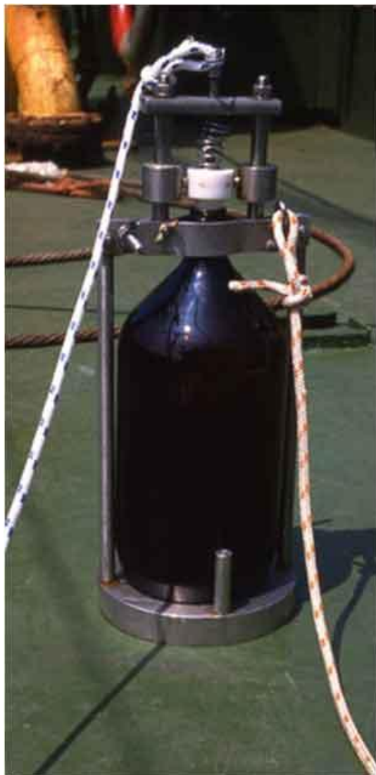
Figure 2.7 – typical bottle used for depth sampling
