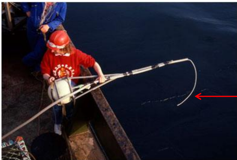
Figure 2.31 – Kevlar sampling tube
