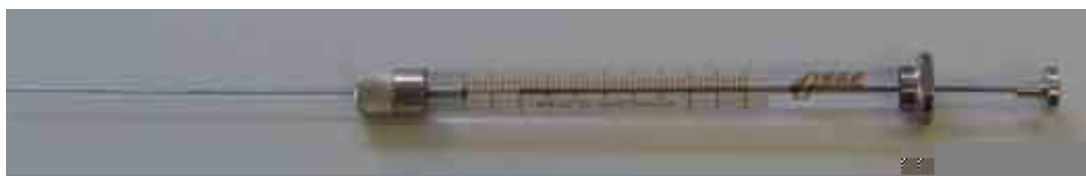
Figure 7.4 - photograph of a microlitre syringe used to inject samples manually into the gas chromatograph
