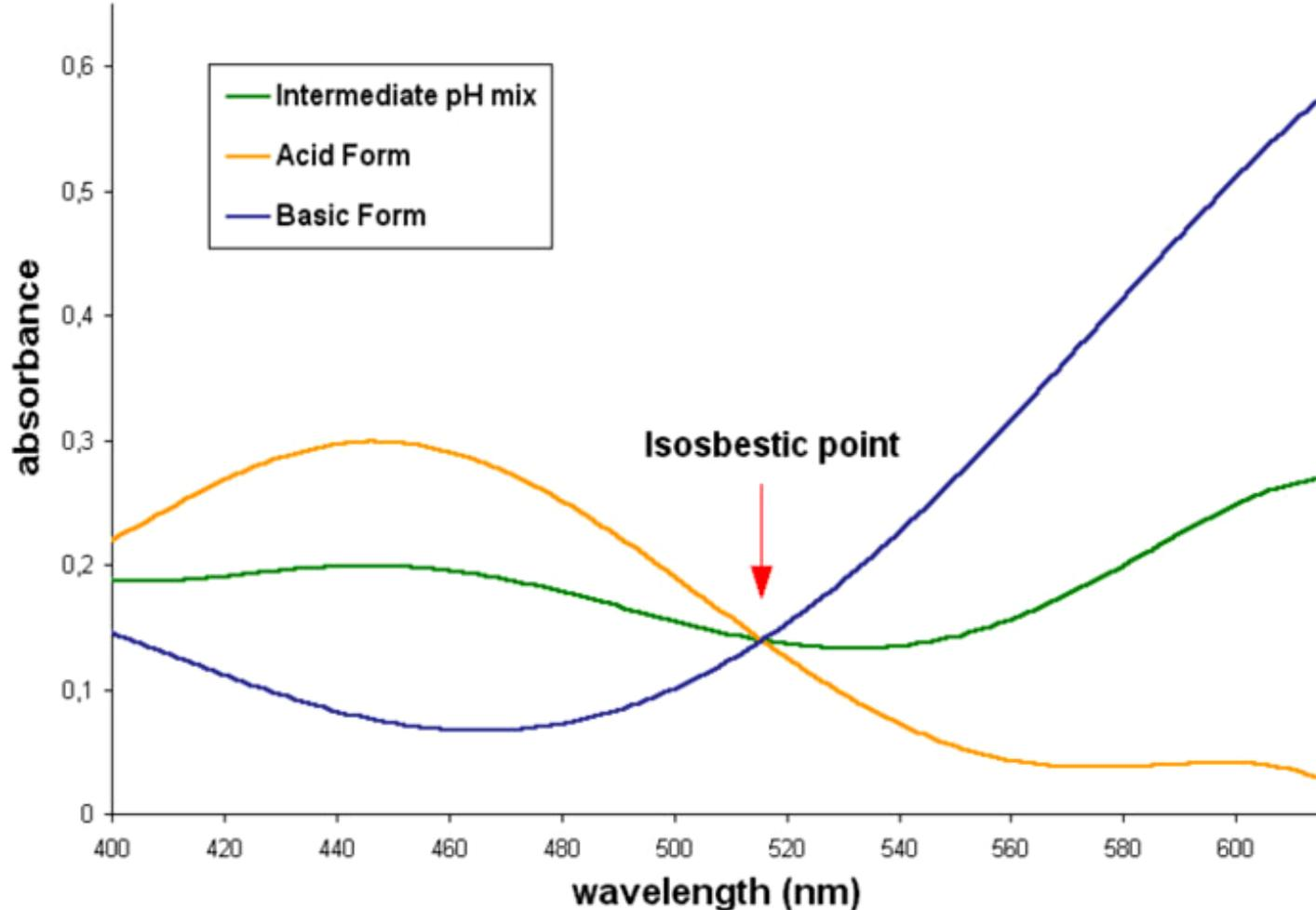
The figure shows the absorption spectra of bromocresol green in acidic, basic, and neutral solutions. The acidic and basic forms of this dye have quite different spectra, but at about 515 nm their  $\epsilon$  values are equal, so the absorbance of a given solution at that wavelength is the same at all pH values. [http://en.wikipedia.org/wiki/File:Bromocresol\\_green\\_spectrum.png](http://en.wikipedia.org/wiki/File:Bromocresol_green_spectrum.png)
