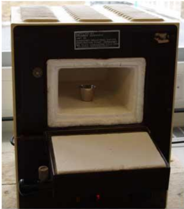
Figure 3.12 – typical small muffle furnace
