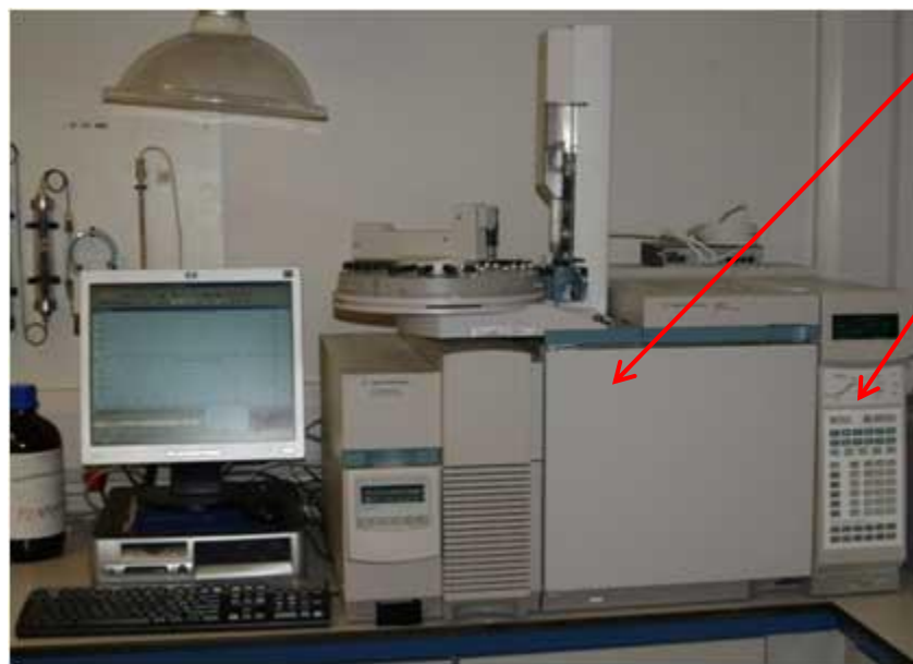
Figure 3.14 – typical gas chromatograph with mass spectroscopy detector
