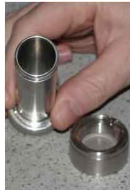
Figure 3.7 - stainless steel extraction cell
