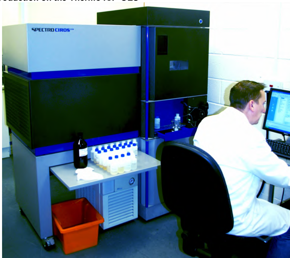
Spectro Ciros ICP-AES designed in the late 1980s is a much larger instrument than those designed today.
