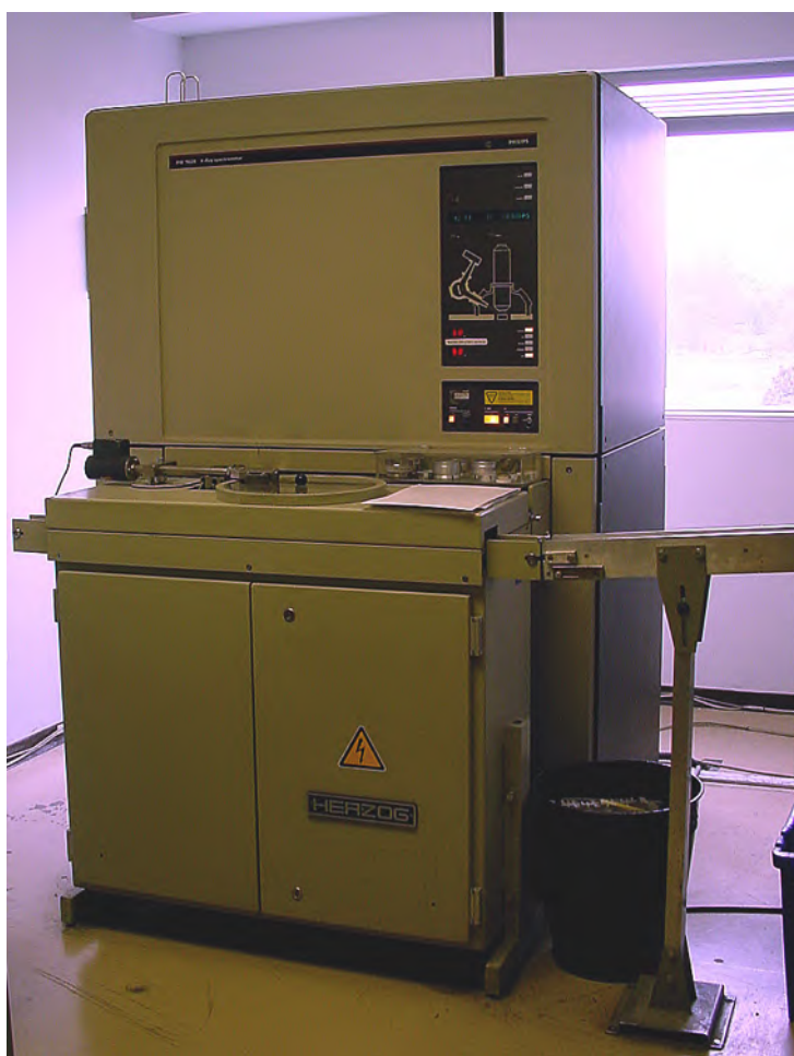
Automated XRF at a cement works
