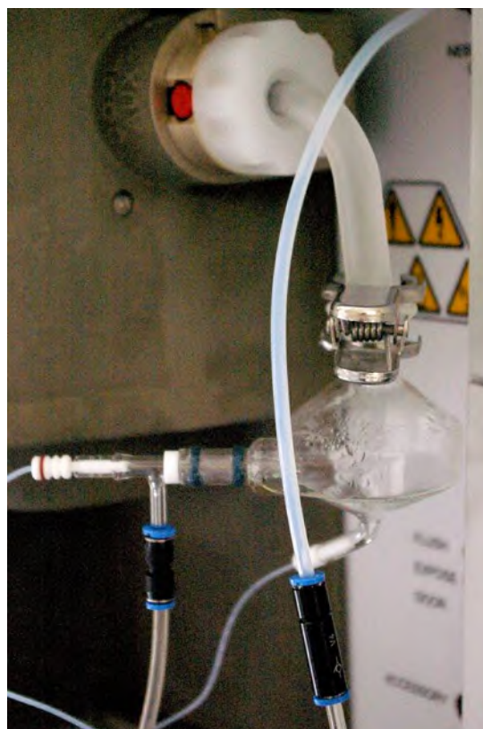
Nebuliser and spray chamber of the Thermo ICP-OES
