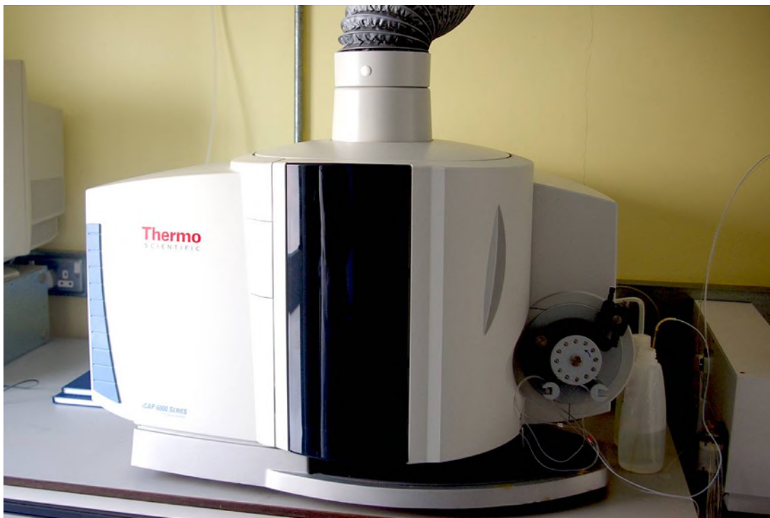
Thermo ICP-OES is a typical example of the modern bench-top instruments
