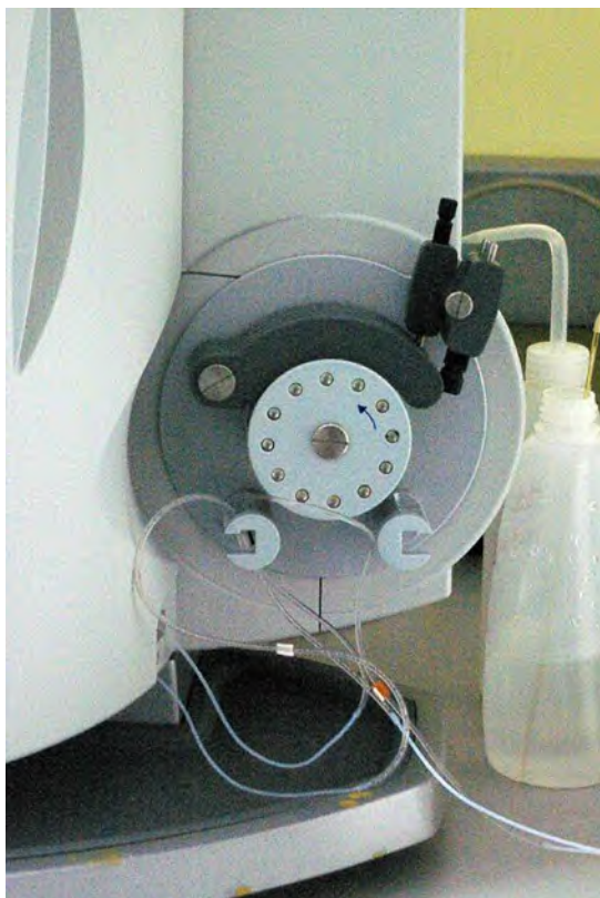
Peristaltic pump for sample introduction on the Thermo ICP-OES
